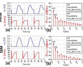
(a) **Simulated** Time domain waveforms: on the left, at the top the switch voltage,  $v_s$ , below, the current,  $i_s$ . (b) On the right the FFT of the  $P_{OUT}$ .
