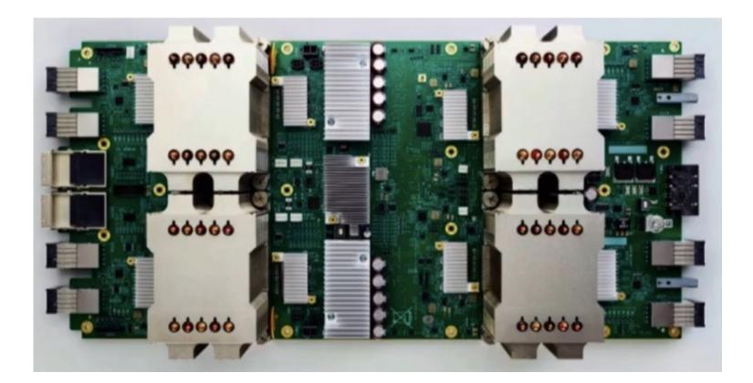
Google's TPU2 : training and inference in a **180 teraflops<sub>16</sub>** board (over 200W per TPU2 chip according to the size of the heat sink)
