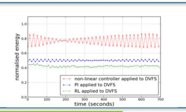
Up to 44% energy reduction, wrt. state-of-the-art (proportional-integral and non-linear controllers)
