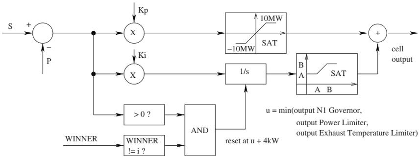
**Fig. 12.** Elementary cell used for the construction of turbogas controller subsystems: N1 Governor, Power Limiter, Exhaust Temperature Limiter. Cell Inputs: S, P, WINNER. Cell Parameters: i, A, B. Known Constants: Kp, Ki (from [10])
