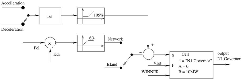
**Fig. 13.** Turbine Rotation Speed Controller (N1 Governor). The switches Acceleration/Deceleration, Network/Island change the controller mode. Their settings are chosen by a higher level controller or by the human operator. Kdr is a known constant (given to us in [10])
