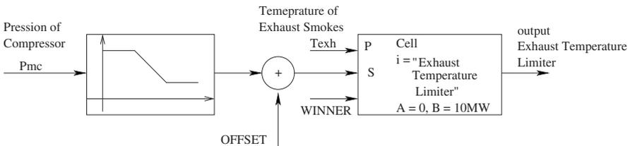
**Fig. 15.** Exhaust Smoke Temperature Controller (Exhaust Temperature Limiter)
