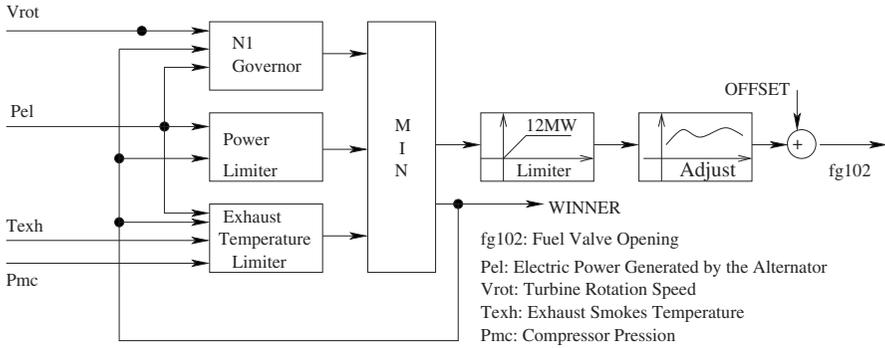
**Fig. 11.** Turbogas fuel gas valve controller.
